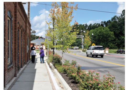
Even in narrow spaces, narrowing traffic lanes and additions of landscaping buffer pedestrians from traffic and calm traffic to safer speeds. (Smart Growth America)
